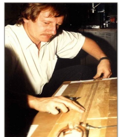
Early version of a spine coil movable beneath the patient, developed in Würzburg during the early phase of MRI development (Noras Medizintechnik).
